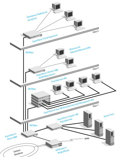
In larger enterprise network environments, the SuperStack II Hub 100 can be used as a scalable, stackable platform enabling users to increase port density, enhance system reliability and add SNMP management. The addition of Ethernet/Fast Ethernet switches and a high-performance bridge/router can provide 100Mbps performance across the network site.
